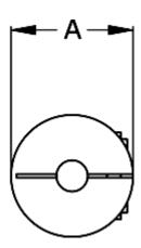
A = 110 D1 = 60 D2 = 60 L = 105 Nom. torque NM (Tkn) = 300
